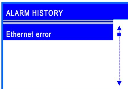
In this submenu item, the history of the occurred error messages can be repeatedly displayed. Also, you can receive more information about the corresponding error such as the date and the time. When they occur, error messages are confirmed with the operating button *Back*.
