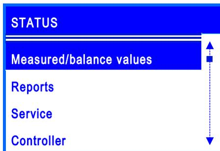
The menu item *Status* contains submenus which allow to look through all measured/balance values, temperatures and flow rates at the sensors, relay states, operating times, heat quantity, tap performance as well as error messages. In addition, the current firmware is displayed at the item *Controller*.
