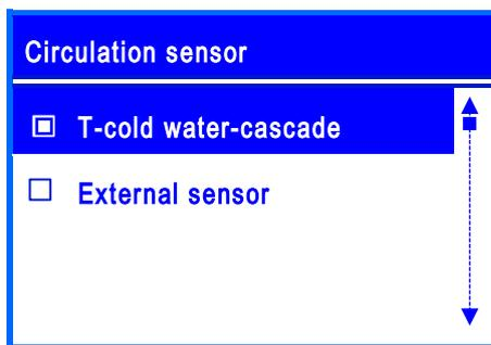
The special characteristic of the temperature control at the cascade is the selection of a new sensor which is called *T cold water cascade*.
