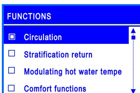
In the example, the ticked check box indicates that the function *Circulation* was activated.
