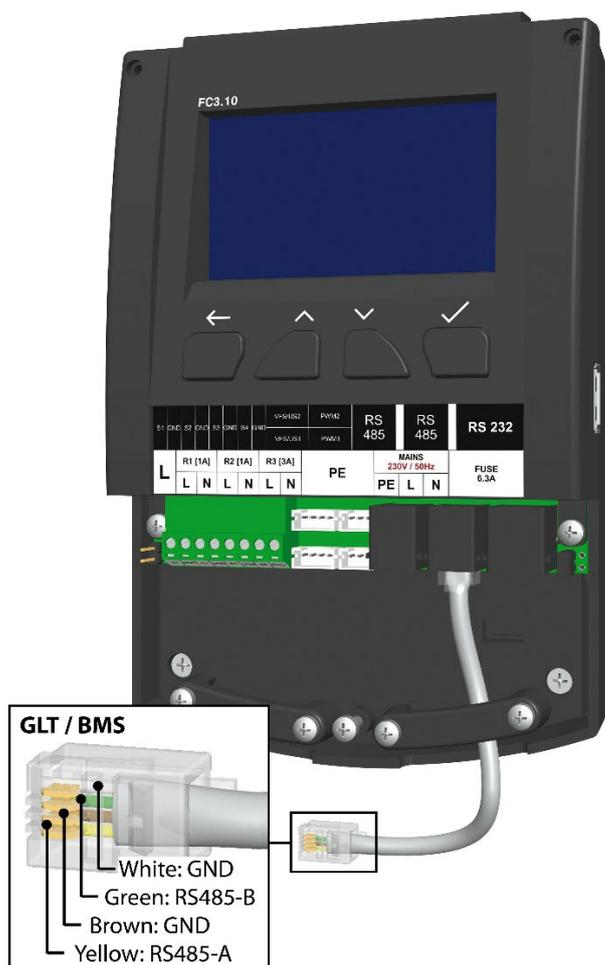
If the connection to the BMS is meant to be realised via a clamping connection, please consider the pin assignment of the communication cable.
