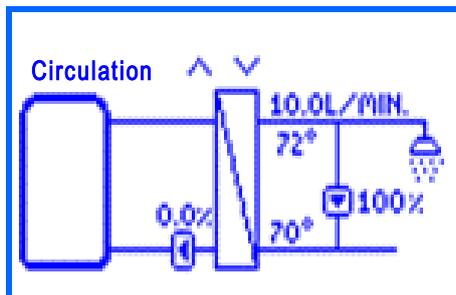
In this menu item, you can set the PWM signal (rotation speed) of the circulation pump with the operating buttons *Upwards* and *Downwards*. With the setting, the flow in the circulation line is modified, and consequently the temperature difference between inlet and outlet.
