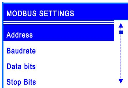
The address is a personal allocation number of the FC3.10 controller (server) within the bus, which the BMS addresses to during the communication.
