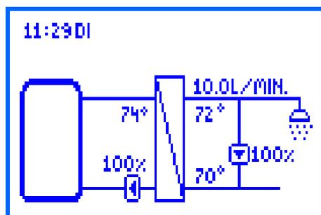
By means of a circulation function, the drinking water in the circulation line is heated to the desired nominal temperature. The designated circulation pump is actuated by the controller via the PWM 2 connection.
