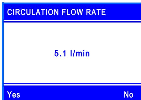
Please confirm the current flow rate which is currently circulated in the circulation mode (no active withdrawal) by the confirmed setting.
