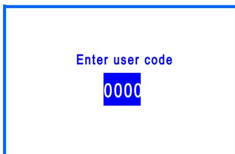
In this menu, you can enter the user code. According to the entered code, a different access to the setting area of the controller is possible.
