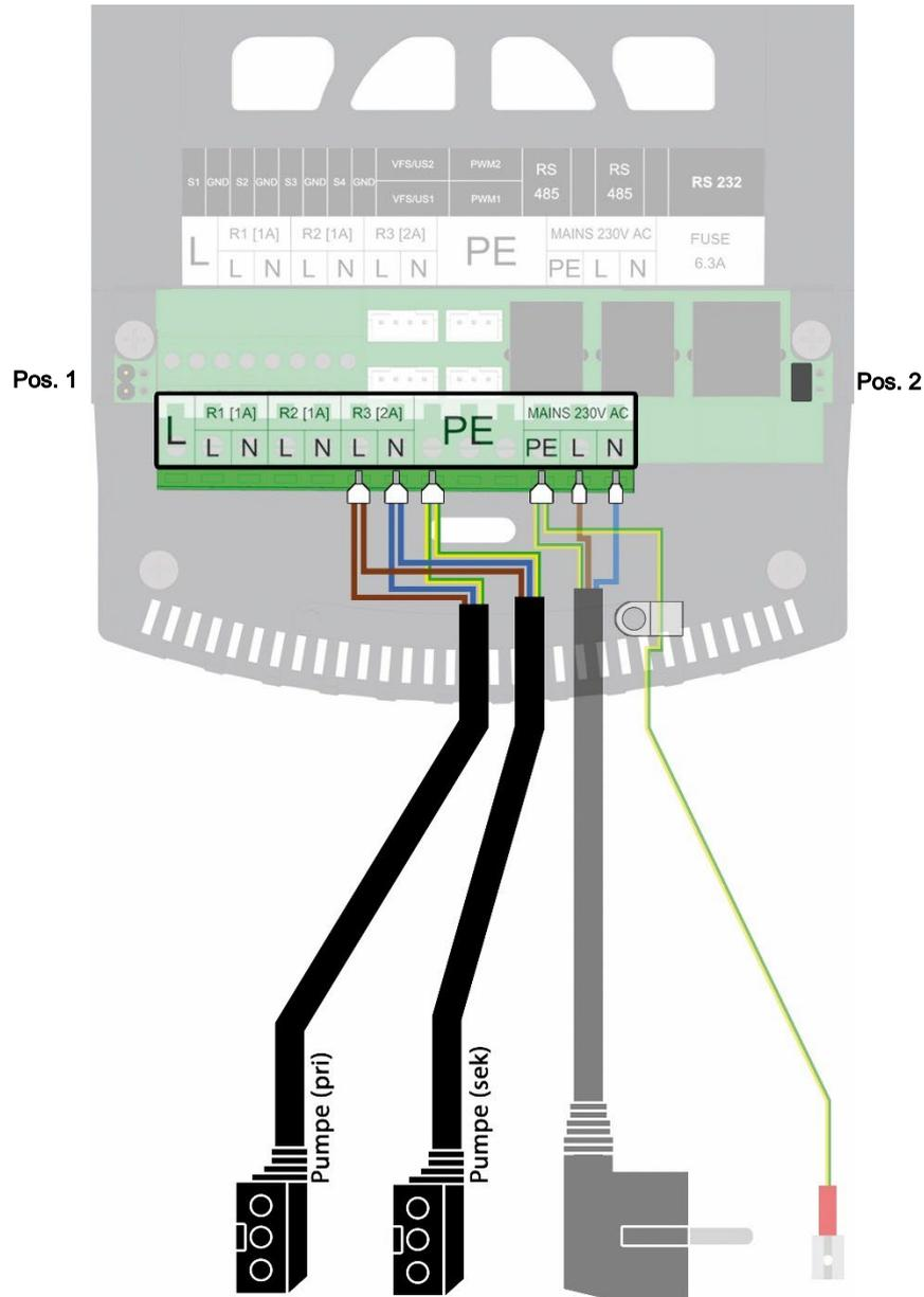
6. For the first and last participant of the Modbus communication, the jumpers must be placed in position 2 (see upper illustration). Place the jumpers as follows:
