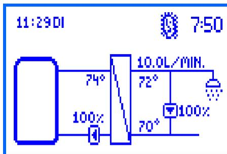
Bigger DHW systems are thermally disinfected in order to kill dangerous germs (such as legionella bacteria) in the system. For this, the domestic hot water module can provide higher hot water temperatures.
