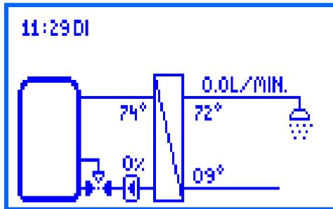
This function serves to improve the temperature stratification in the storage tank or to avoid a temperature mix. In the return can be considerable temperature differences (for example, with an existing circulation). Therefore, the return is connected to the storage tank via a three-way valve.
