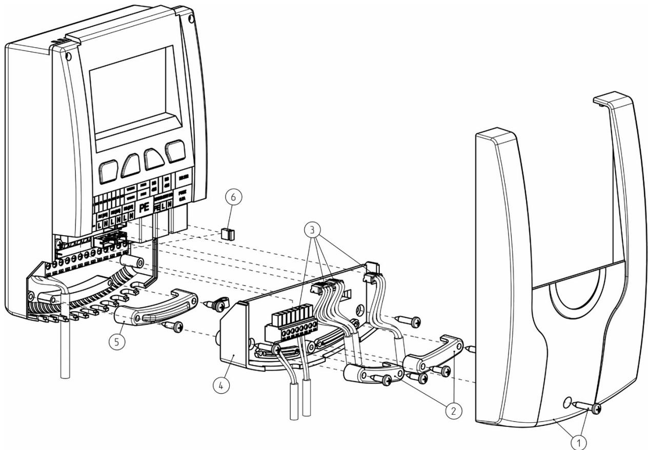
1. Remove the white front panel of the controller (1).
