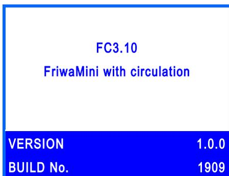
Display of the current software version and the domestic hot water module which was selected during commissioning.
