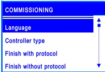
To complete the commissioning at the servers, confirm the items *Finish with protocol* (for this, a USB flash drive must be connected to the controller) or *Finish without protocol*.
