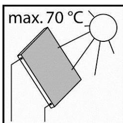
Under the influence of solar radiation, the collectors can get very hot. The solar fluid in the circuit can heat up to more than 100 °C. Only flush and fill the solar circuit if the collector temperatures are below 70 °C.
