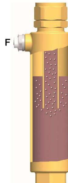
The air separated from the solar fluid is collected in the upper part of the Airstop and can be released at the vent plug [F].
