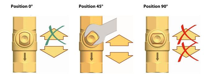
Check valve is operating, **flow** only in flow direction.
