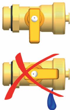
18. Remove the hoses of the flush and fill station and screw the sealing caps on the fill and drain valves.
