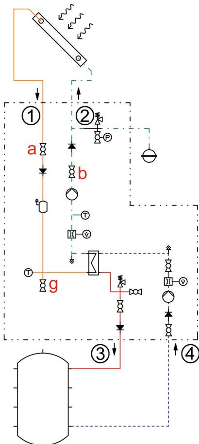
1. Close the ball valves [a|b] and release the solar fluid at the fill and drain valve [g]. Make sure that the solar fluid is collected in a heat-resistant container.
