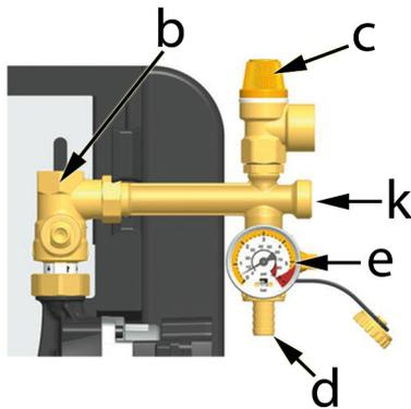
8. Assemble the safety group consisting of safety valve [c], fill valve [d] and pressure gauge [e] on the connection of the return ball valve [b].
