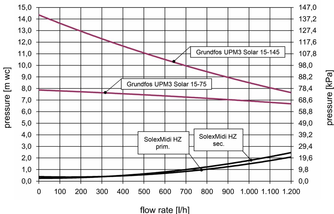
7.4 Pressure drop and pump characteristic curves SolexMaxi HZ
