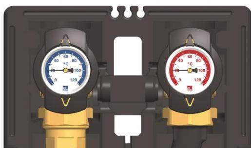
4. The thermometer ball valves are respectively equipped with 2 sleeves G $\frac{1}{4}$ " which are sealed with a plug. These sleeves can be used to mount the temperature sensors of the heat flowmeter.
