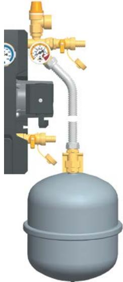
1. Connect the stainless-steel corrugated hose to the safety group. Do not forget to insert the seal.
