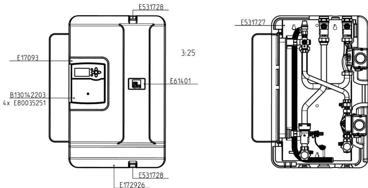
8.3 Insulation and controller tank heat transfer module Maxi (6436465)
