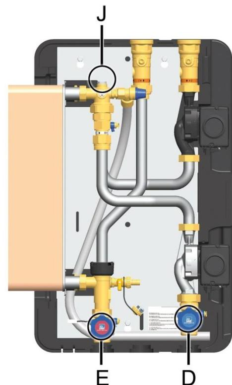
8. Open a withdrawal point for domestic hot water (for example a tap) with a flow rate of at least 10 l/min and let the water run for about 2 minutes to vent the secondary circuit. Close all withdrawal points of the secondary circuit afterwards.
