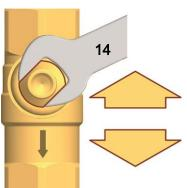
Check valve is not operating, flow in both directions.
