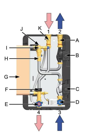
Example: Tank heat transfer module Maxi
