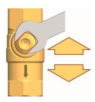
Check valve not operating, flow in both directions.
