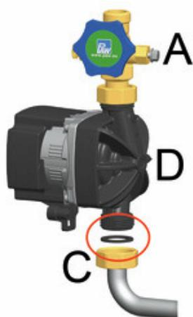
5. Coming from the left, mount the pump [D] with the piston valve [A] to the short limb of the pipe [C]. Do not forget to insert the gasket.
