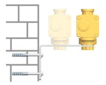
If possible, choose the largest distance to the wall. It is thus easier to mount the insulation of the distribution manifold.
