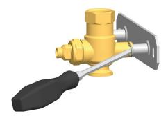
To remove the boiler charging set from the mounting plate, push the clips sidewards with a screwdriver. The boiler charging set can then be pulled forwards (consider the tubing!).
