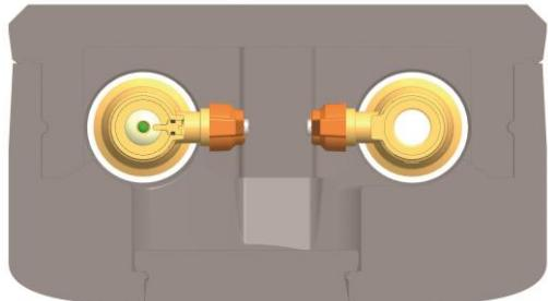
3. The handles of the pump ball valves must be turned inwards in order to close the front insulation (see figure on the left).
