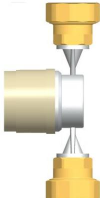
1. Dismount the adapter pieces of the adapter pipe first and mount them on the heat flowmeter.
