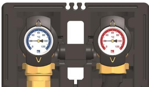
5. The thermometer ball valves are respectively equipped with 2 sleeves G $\frac{1}{4}$ " which are sealed with a plug. These sleeves can be used to mount the temperature sensors of the heat flowmeter.
