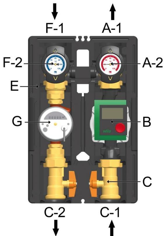
The fitting for heat flow meter is mounted in the return line of the heating circuit. The flow sensor for the heat quantity measurement can be mounted in the flow thermometer ball valve [A-2] or in connections required on site by using one of the enclosed reducers.
