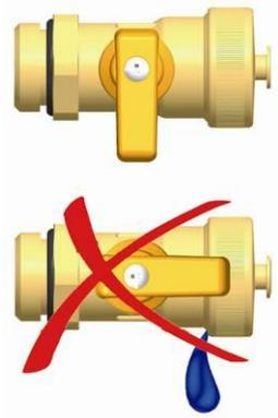
25. Remove the hoses of the flush and fill station and screw the sealing caps onto the fill and drain valves.
