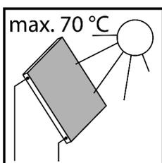
Under the influence of solar radiation, the collectors will heat up considerably. The solar fluid in the solar circuit may heat up to more than 100 °C. Only flush and fill the solar circuit when the collector temperatures are below 70 °C.
