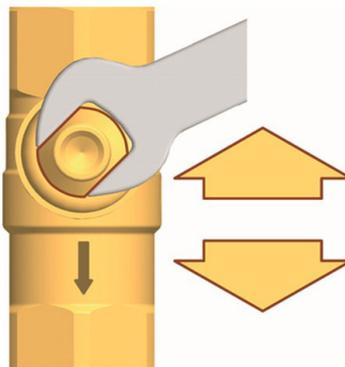
Check valve not operating, **flow in both directions.**
