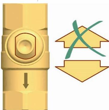
Check valve is operating, **flow only in flow direction.**
