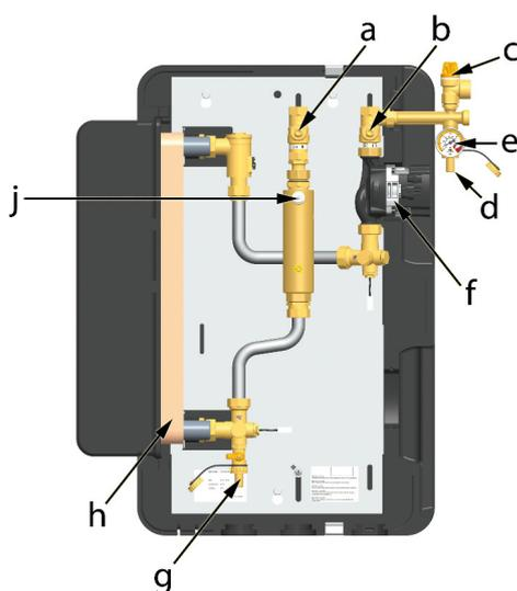
8. Close the drain valve [g] with the filling pump running and increase the system pressure to approx. 5 bars. The system pressure can be read on the pressure gauge [e].
