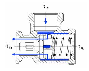
The thermal valve shuts off the connection to the buffer tank, as long as the water in the boiler circuit is colder than the opening temperature of the thermal control valve.
