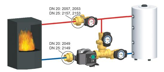
Mounting version 1B permits to easily isolate the heat generation system without further shutoff valves. Necessary accessories: gasket, fitting, pump fitting
