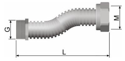
Flexan is a fitting system for flexible connections, it permits to quickly compensate length differences and offsets, for example for the assembly or exchange of radiators. Stretchable by 75 %. Not suited for dynamic loads!
